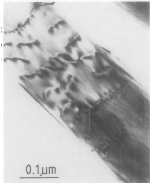
FIG. 5. Dislocation-type defects in a lath of \text{Cs}_2\text{Ti}_5\text{O}_{11} after lengthy storage, [001] projection.
