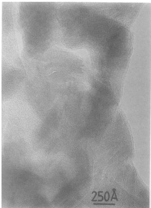
FIG. 2. Paracrystalline character of \text{Cs}_2\text{Ti}_3\text{O}_{11} after deposition from a slurry formed by grinding freshly prepared material in water.
